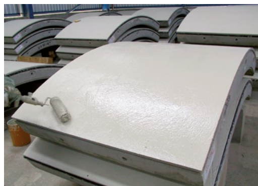
Fig. 8.4.4: Immediately following curing in a steam channel, the concrete surface of tunnel lining segments is coated with water-based epoxy emulsion that is absorbed even into the smallest pores, thereby generating a sealed, protective coating.
